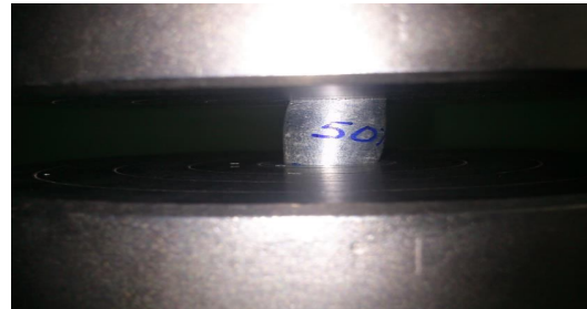
Composite specimens showing bulge profiles at various deformation stages under compression testing ( H_0/D_0 = 1.0 & H_0/D_0 = 1.5 )
