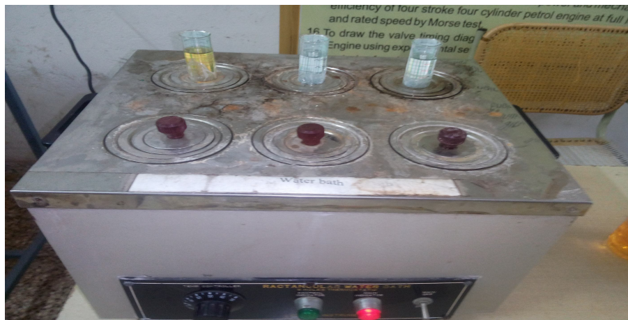
Fig : Experimental setup for measurement of diffusivity.
