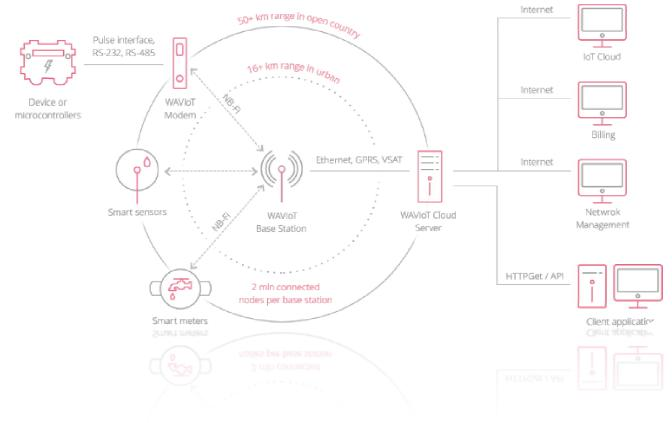
The solution is well suited for worldwide deployments, supporting radio hardware and compliant MAC architectures in 915 MHz, 868 MHz, and 433 MHz ISM bands, as well as other sub-GHz license-free spectrum bands.
