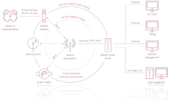
The solution is well suited for worldwide deployments, supporting radio hardware and compliant MAC architectures in 915 MHz, 868 MHz, and 433 MHz ISM bands, as well as other sub-GHz license-free spectrum bands.
