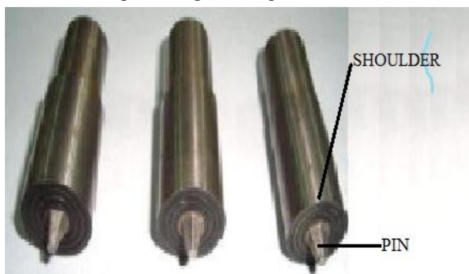
Fig 3.3 Tool used in Friction stir welding
