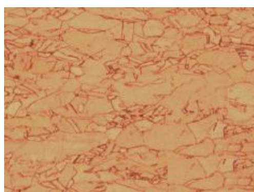
Fig 4.2 (f). Microstructure of HAZ of RS
