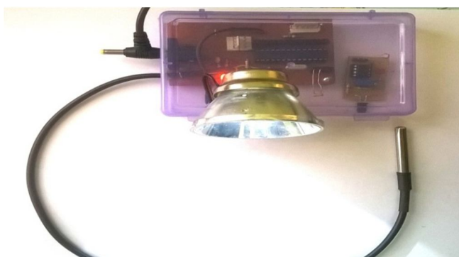
Fig 3 Li-Fi based implemented Wireless Sensor Node
