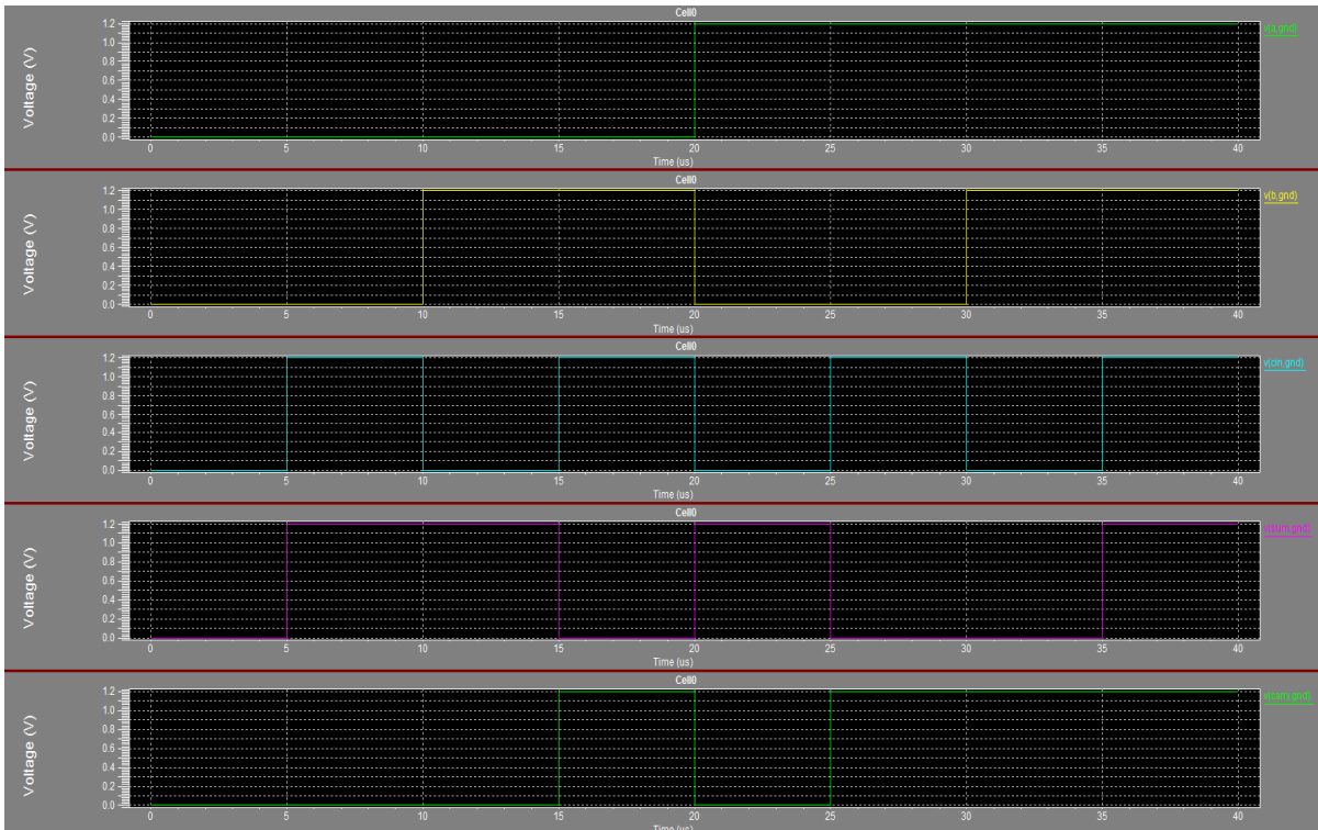
Fig.11 W-edit output waveform of 10T Full adder.
