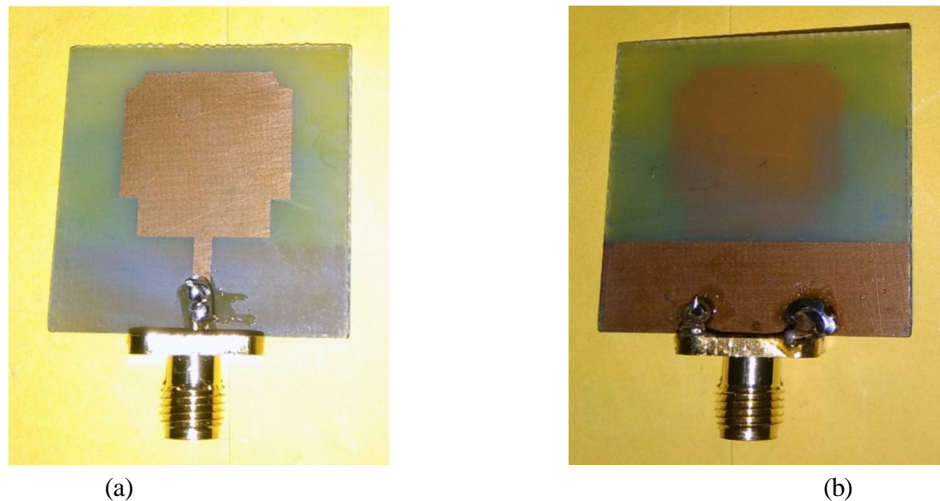
Figure 6 Single Element Fabricated Antenna (a) Front view (b) Back view
