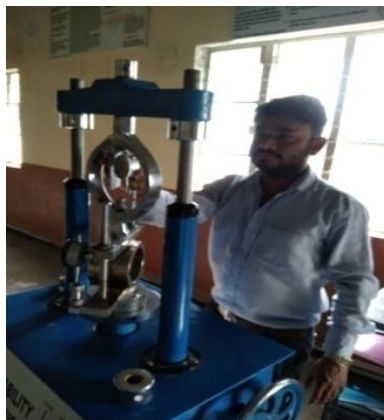
Figure 4.1 Performing Marshall Test
