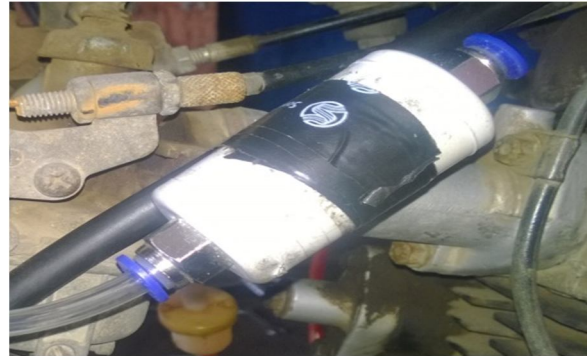
Fig1(b) MOISTURE FILTER
