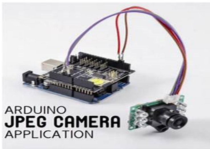
Fig 5: Interfacing Of Arduino With Web Camera
