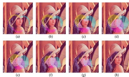
Fig.5. Illustration of pixel processing order in watermark embedding and removal. (a) - (d) intermediate results of image watermarking when 25%, 50%, 75%, and 100% of the watermark pixels have been processed, respectively. (e) - (h) intermediate results of image recovery when 25%, 50%, 75%, and 100% of the watermark pixels have been recovered, respectively.
