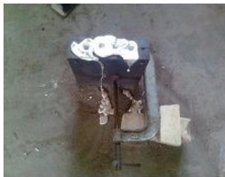
Figure 2: Solidification of Composites in Metallic dies
