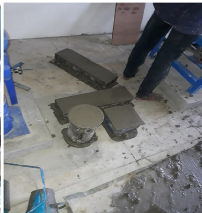
Fig. 7. Casting of Specimens Curing
