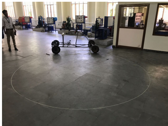
Figure 8.1: Turning circle of the prototype
