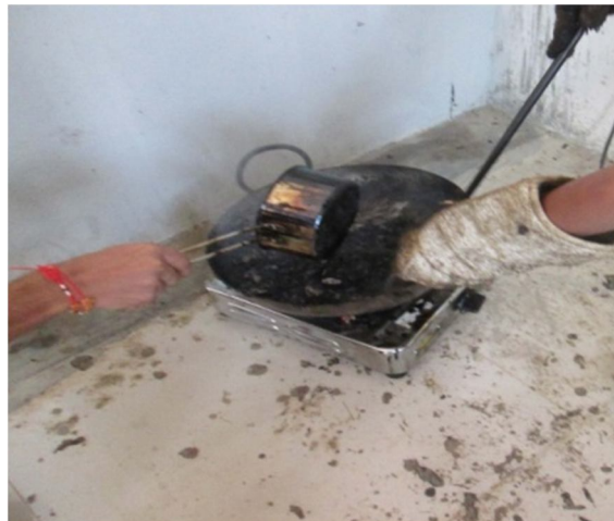
Fig.3Mixing of waste plastic with bitumen
