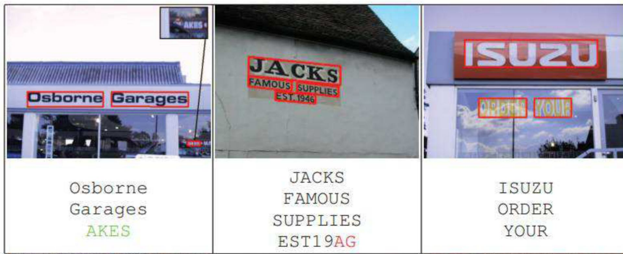
Fig. 8: End-to-end recognition examples of [13]. This is the first real end-to-end system for scene text recognition.
