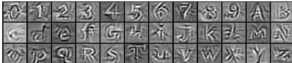
Fig.9 Filters learned from characters in natural images [19]. As can be seen, the learned filters can capture the shapes of the corresponding characters.
