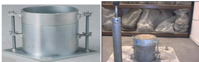
Fig 3.2(a) CBR Mould (b) Compacted Plastic waste strips mixed soil in CBR mould
