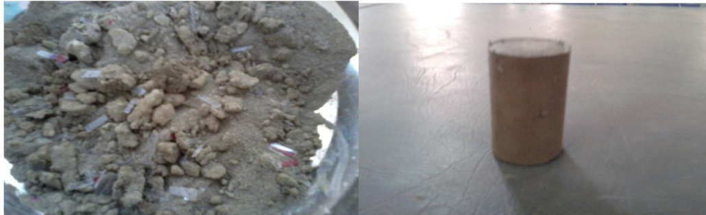
Fig 3.1 (a) Plastic waste strips mixed soil (b) Sample prepared with plastic waste mixed soil
