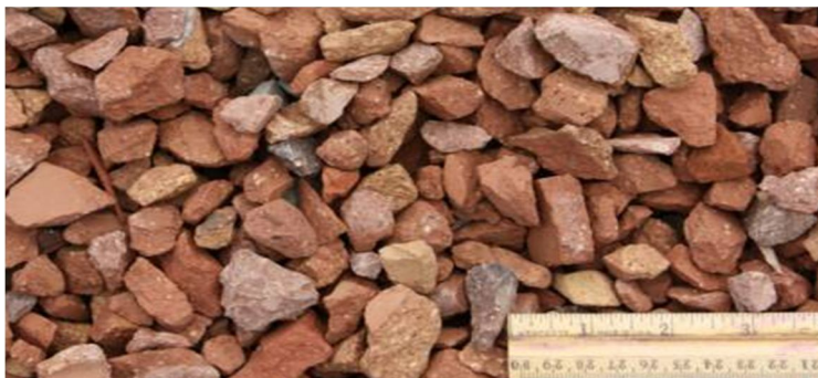
Fig. 1 Broken or crushed brick , specimen : Effective size: 0.15 to 0.35mm Specific gravity: 1.6 approx.
