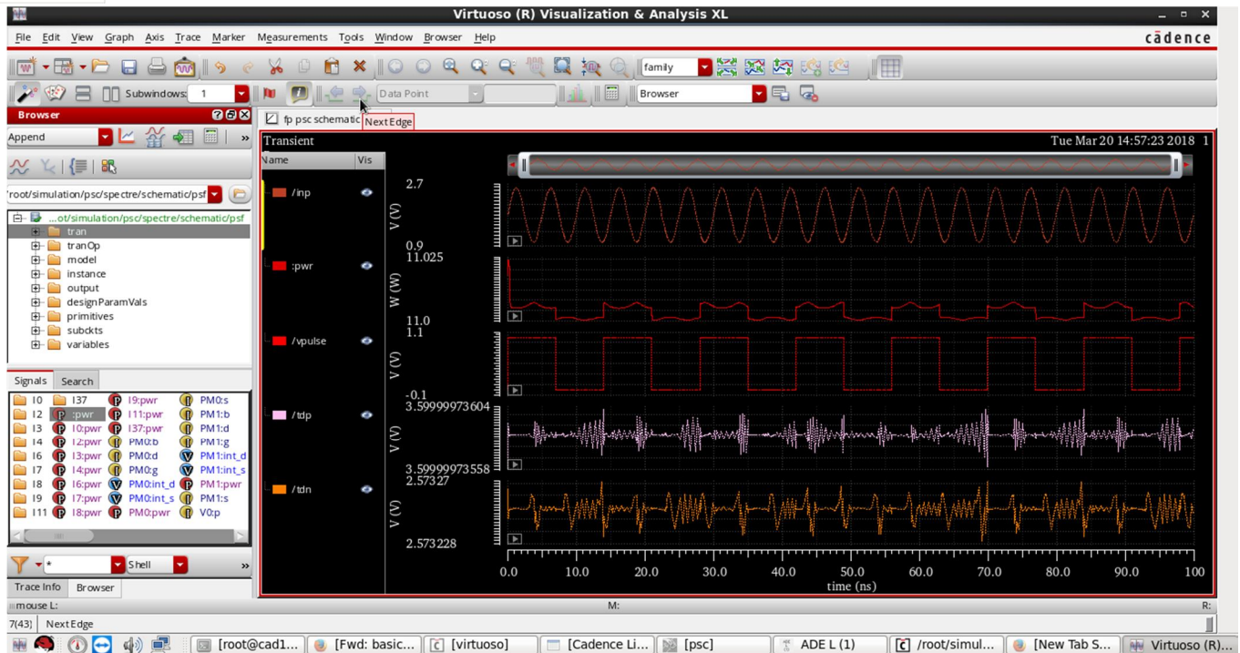
Fig.8 Output waveform of block diagram with dc offset cancellation
