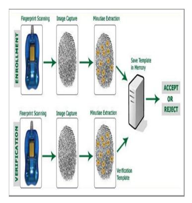
Working can be explained further, This system operates by given a input by the finger print sensor and the matching is done by the finger print module if the input is matched ,the microcontroller generates a signal and it allows the transferring the data from the host computer and the data traveler.
