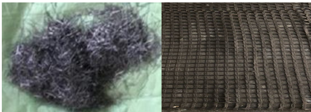
Fig. 1. (a) Hooked end steel fibre; (b) Bi-axial Geo- grid
