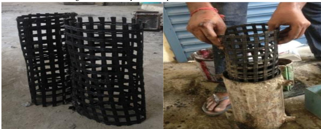
Fig. 2. (a) Tubular form; (b) Inserting the tubular form inside the cylindrical mould.
