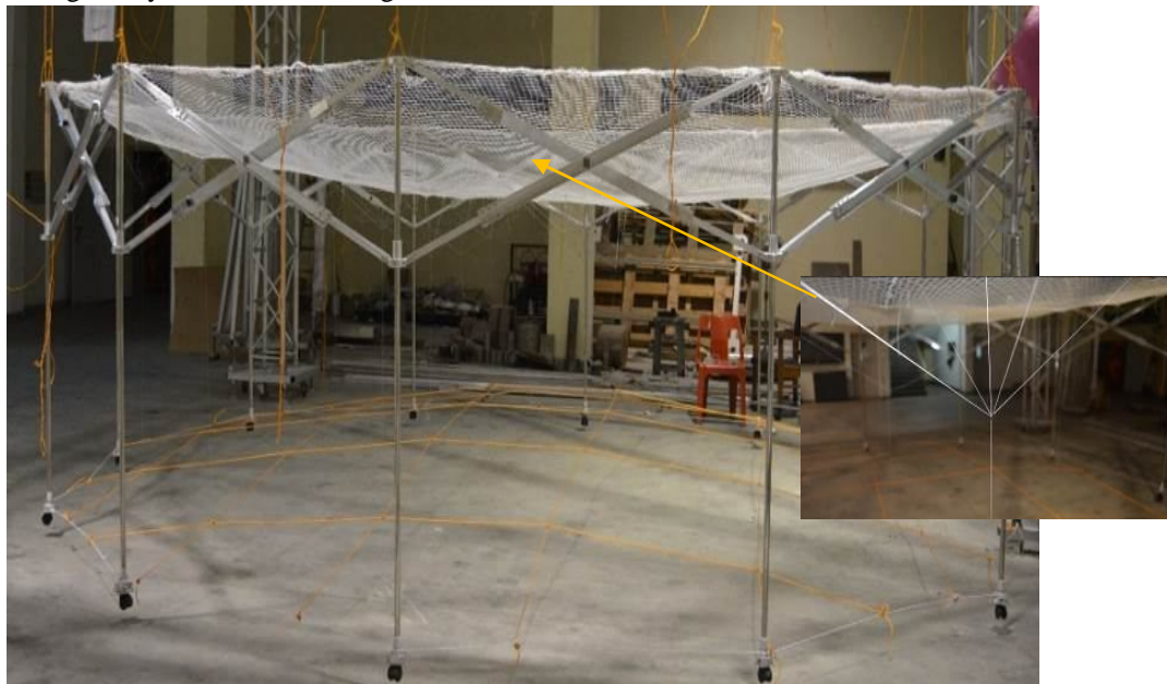
Fig. 4 Shape adjustment using ropes and strings
