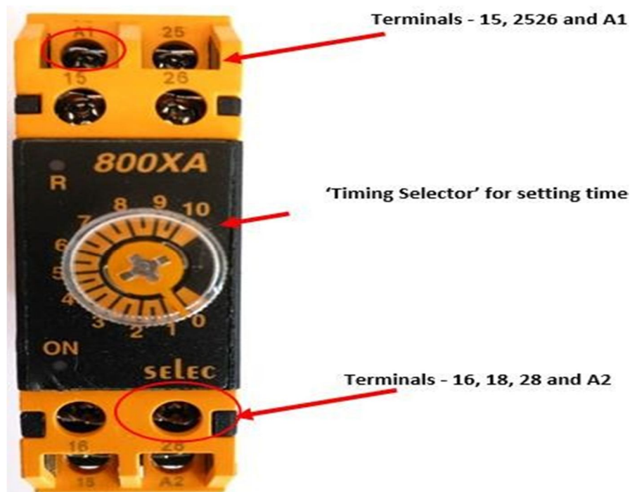
Fig-3: OFF Delay Timer Unit
