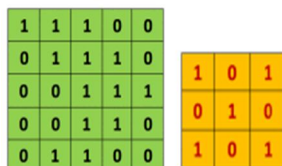
Figure 3.1: 5X5 input image and 3X3 Filter. Source [11]
