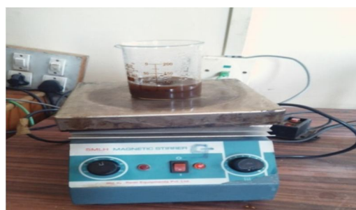
Fig 2: Synthesis of silver nanoparticles by reduction of \text{AgNO}_3 on magnetic stirrer.
