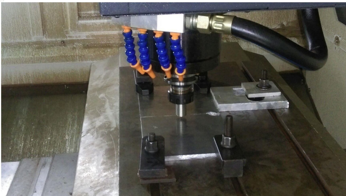
Figure 2: Plates butt welded on the fixture
