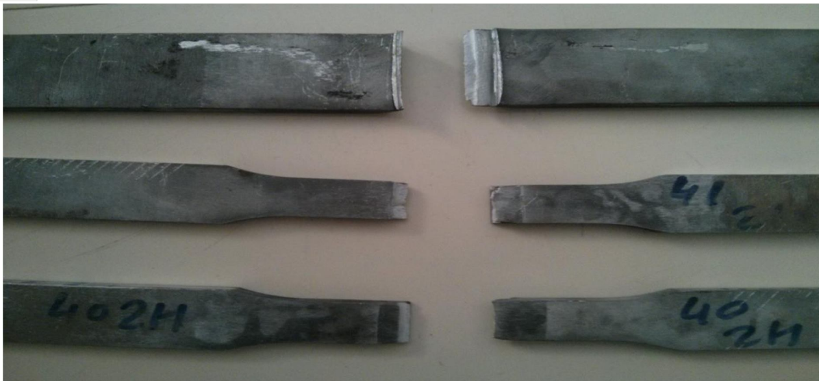
Figure 5: Failure occurrence at the weld zone of the tensile test specimens
