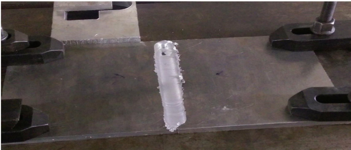
Figure 3: Less formation of flash and chips in the weld
