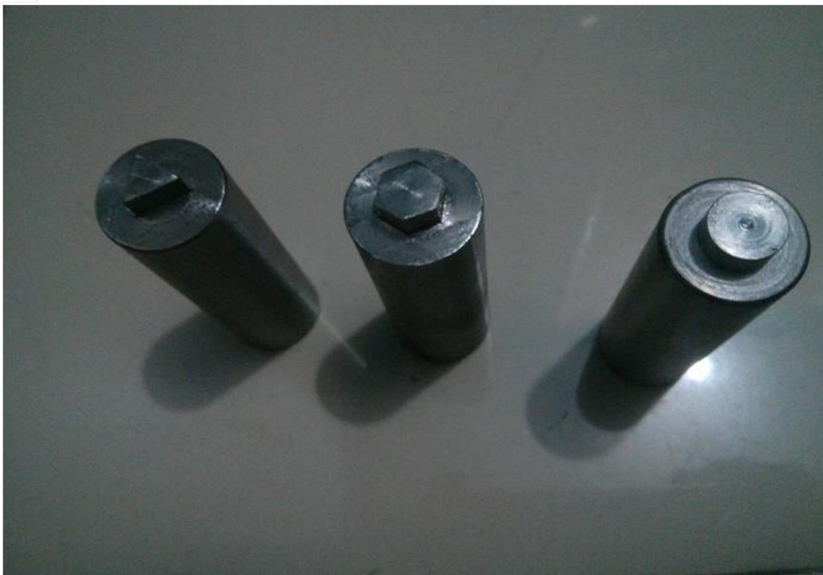
Figure 1: Triangular, Hexagonal and Triangular tool pin profiles
