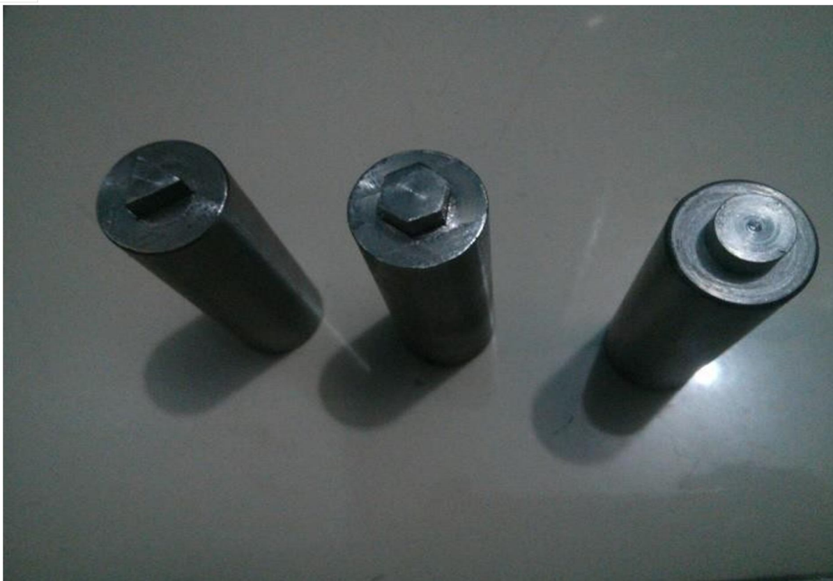
Figure 1: Triangular, Hexagonal and Triangular tool pin profiles
