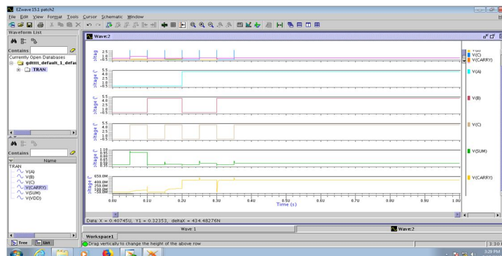
Fig(18) :Wave forms of GDI structured based Full adder
