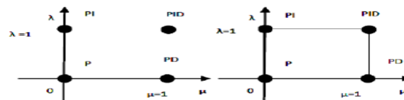
Fig 2.: Fractional-order PID vs classical PID
