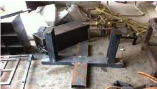
Fig.2 Fabrication of base stand
