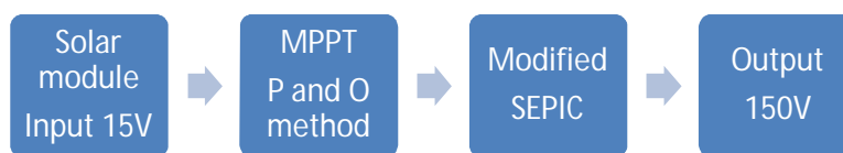
Fig.14 – Block diagram of simulation of modified SEPIC without magnetic coupling
