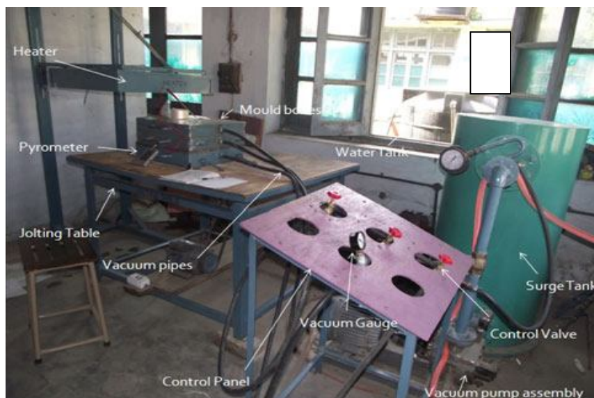
Fig. 2 The schematic view of vacuum moulding.
