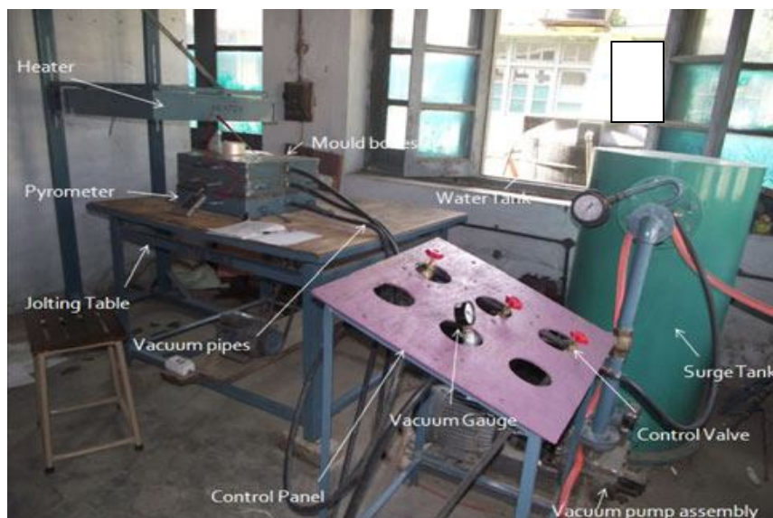
Fig. 2 The schematic view of vacuum moulding.
