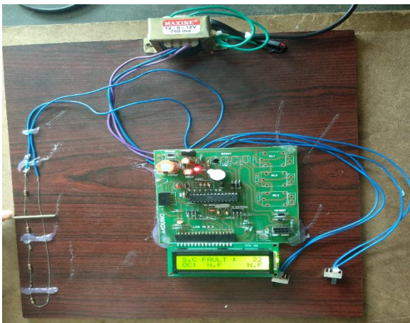
Fig. 7 Short circuit fault
