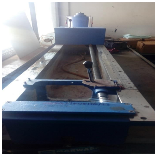
Fig.12 Ductility test apparatus
