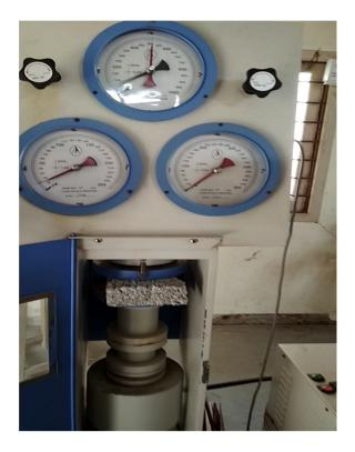
Comperssion testing is done to check the maximum strength the block can withstand here the pervious block can withstand 500KN which is enough to withstand a fully loaded truck on it.
