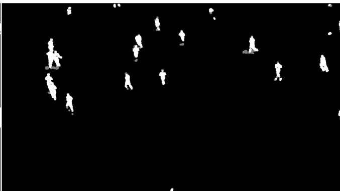
Fig. 4 Morphological Open Operation with 3x3 cell element
