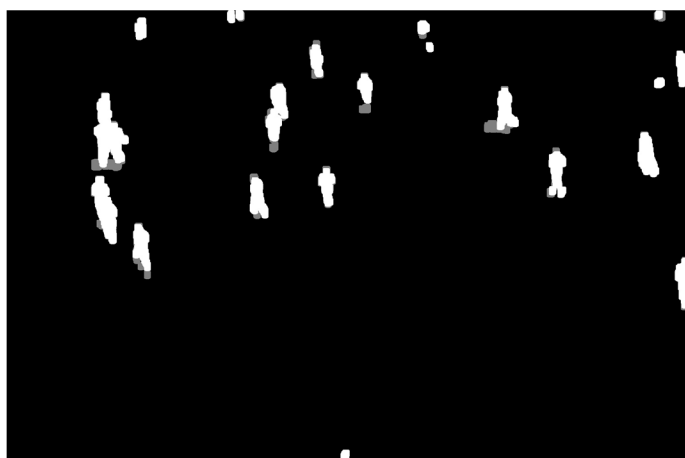
Fig. 5 Morphological Dilation Operation with 50x50 cell element
