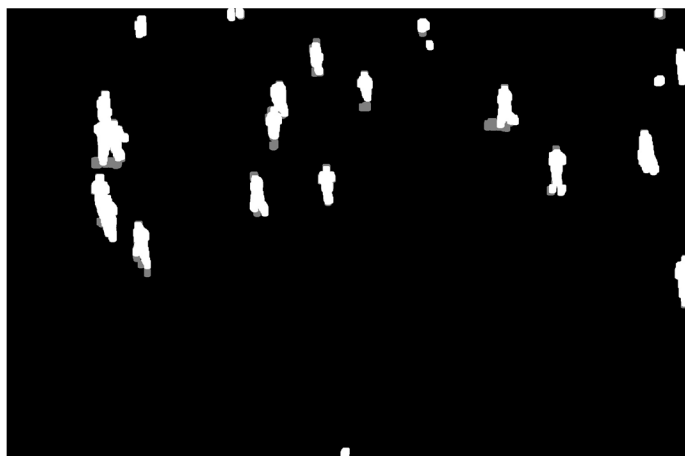
Fig. 5 Morphological Dilation Operation with 50x50 cell element
