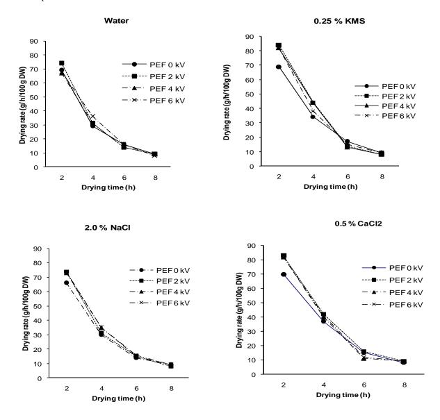
Fig 1: Drying rates of potato slices pre-treated with various chemicals and levels of PEF
