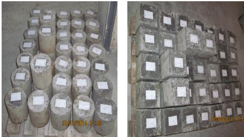
Fig. 2 Test specimens for determining concrete compressive strength according to EN 12504-4:2004
