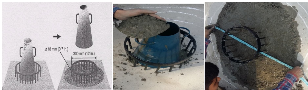
Figure 6: J-Ring Test Equipment
