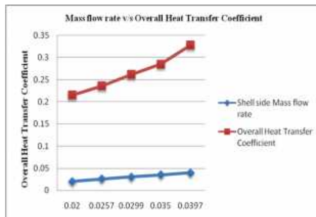
Fig g. Variation of Overall Heat Transfer Coefficient w.r.t Flow rate of the Exchanger.
