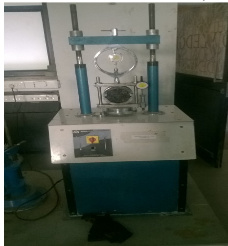
Fig 1 Marshall test apparatus with mould testing (Source –MEFGI highway laboratory)
