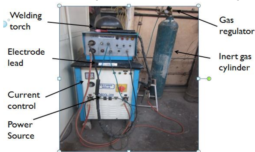
Figure 1: GTAW Setup (Courtesy: Paanchal Weld Workshop, Faridabad)
