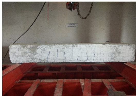
Figure 7 Crack Pattern after loading
