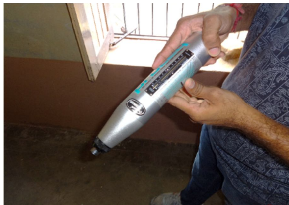
Figure 1 Rebound hammer Test apparatus
