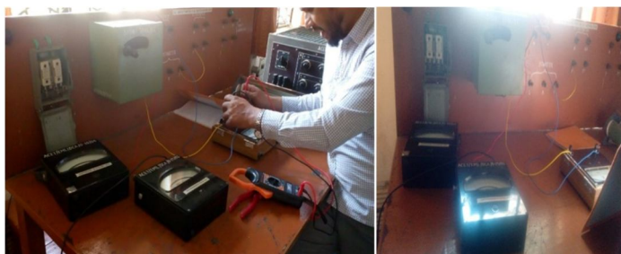
Fig.9 Steel loss estimation setup.
