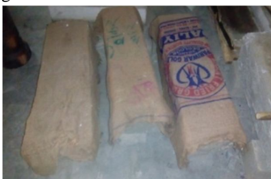
Fig.5 Curing of beams.
