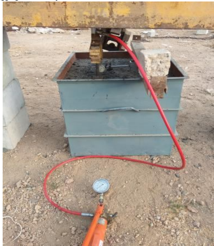
Figure 16 Testing on Geotextile Based Sample
