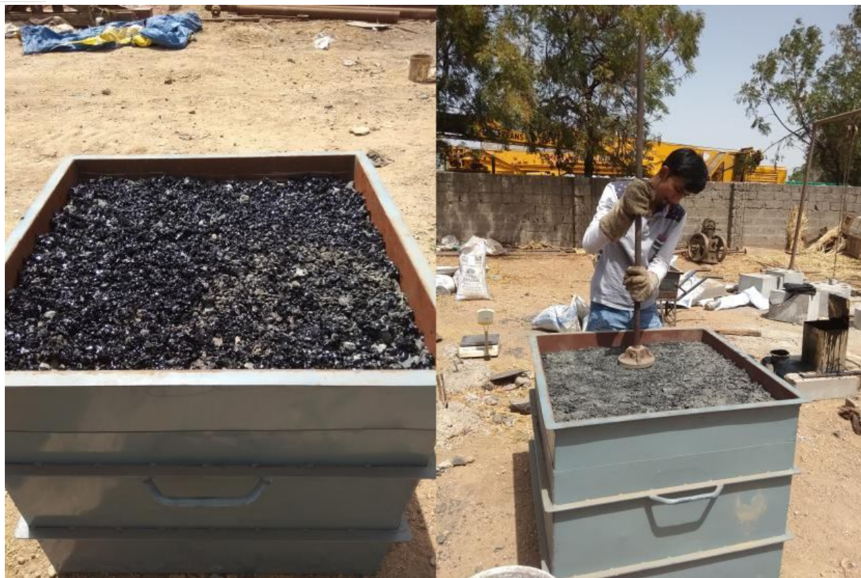
Figure 9 Laying and Compaction of Binder Course
