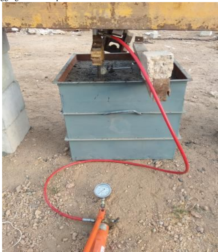
Figure 16 Testing on Geotextile Based Sample
