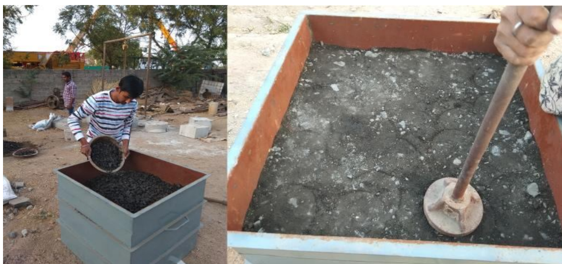
Figure 8 Laying and Compaction of Base course/WMM
