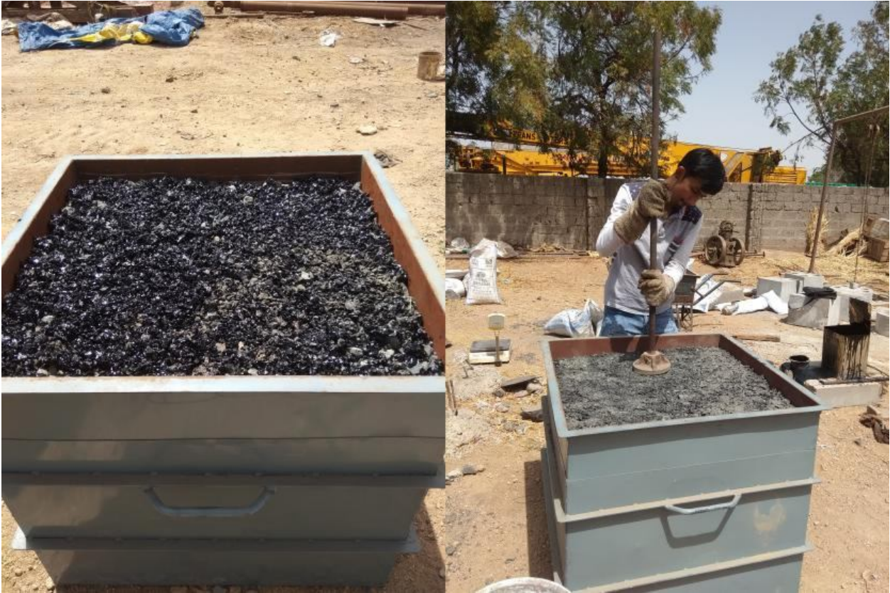
Figure 9 Laying and Compaction of Binder Course
