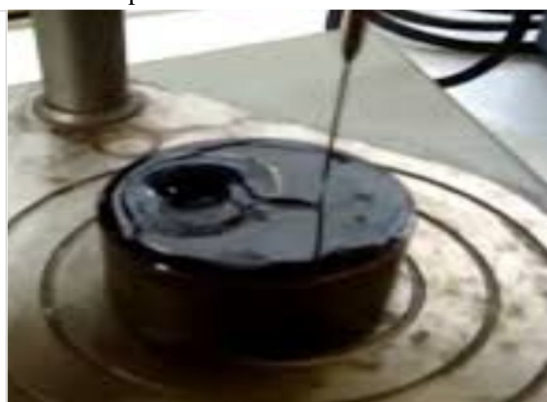
Fig. 5: Assembly for Penetration
