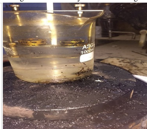
Fig. 6: Assembly for Softening point
