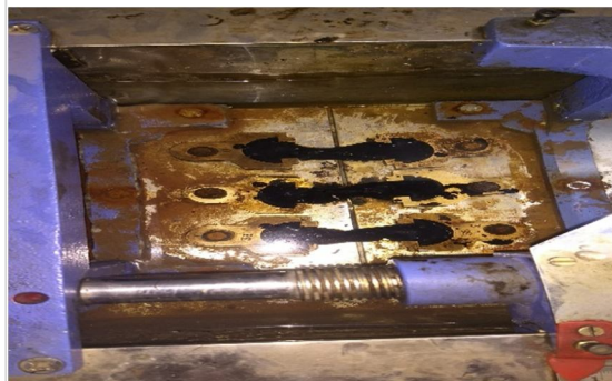
Fig.4: Assembly for Elastic recovery
