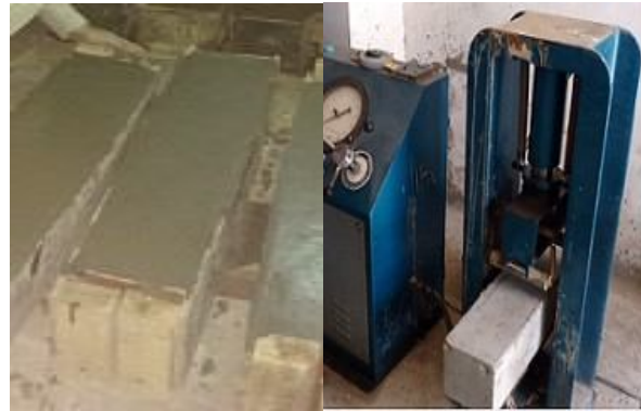
Fig. 14 Casting and testing of beam
