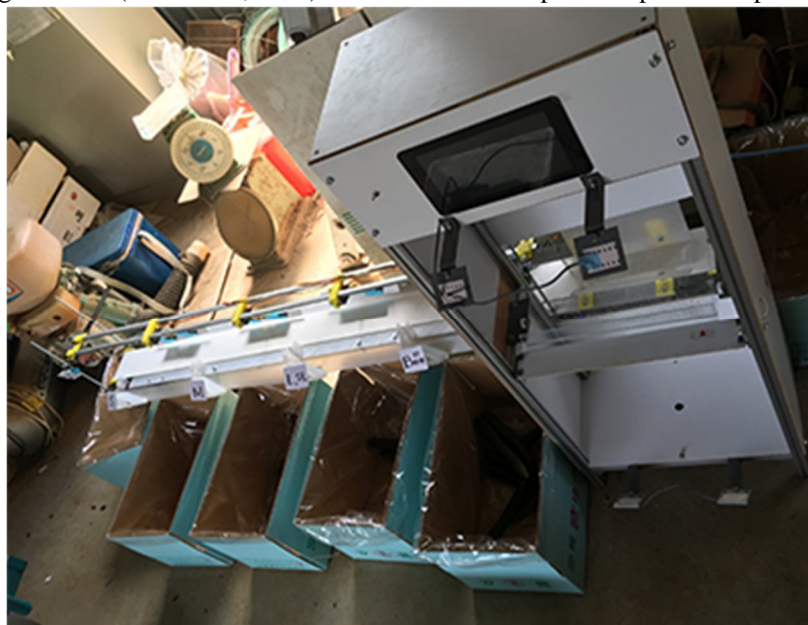
Figure 1. Cucumber sorting machine.
