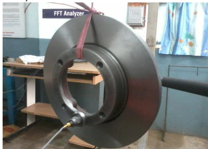
Fig. 13 Accelerometer location
