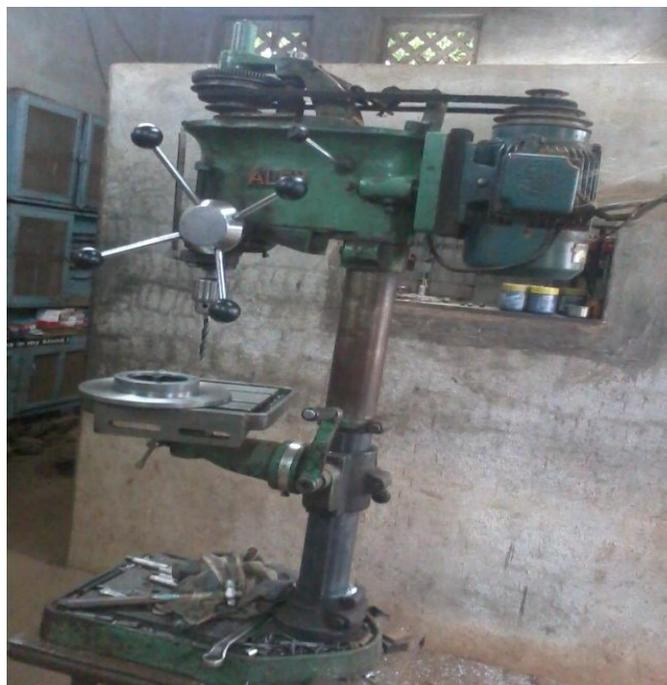
Fig. 10 Vertical axis drilling m/c
