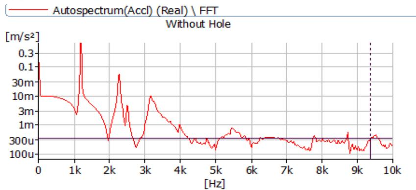
Fig. 16 Acceleration v/s Natural frequency for original disc
