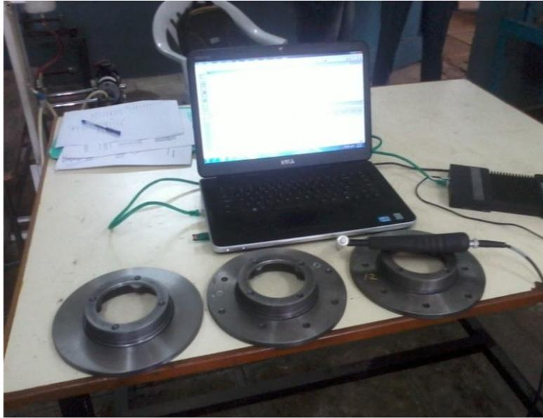
Fig. 15 FFT analyzer setup
