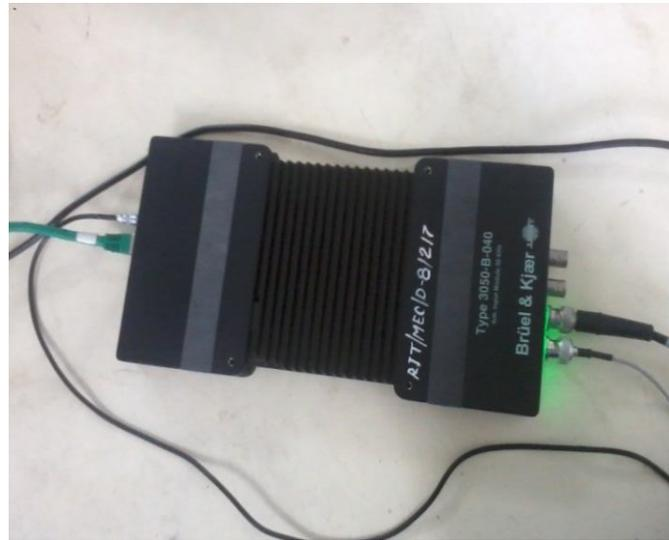
Fig. 12 FFT Analyzer
