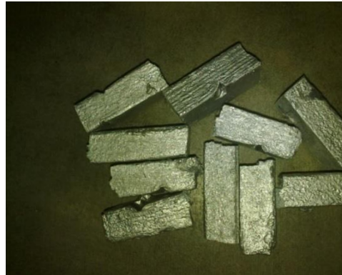
Figure 2 (b). Specimen after the Impact Test
