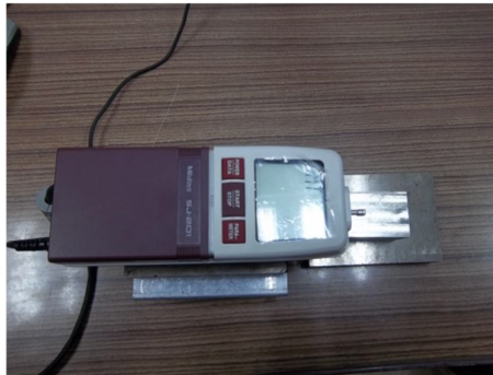
Fig 6.1 Measurement of Surface Roughness - Mitutoyo surf test SJ-200
